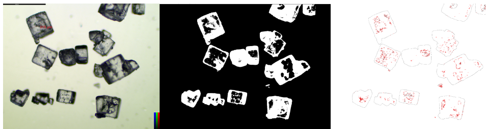
Figure 5: Example of image processing for segmentation & tracing of salt ( \text{NaCl} ) crystals using ImageJ software. Raw image (left) is thresholded to produce binary image (center). Software is then used to produce traces, stored as regions of interest (right).
